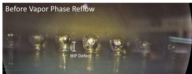
Fig. 4. Two images of solder joints of a BGA/LGA hybrid connector. The left image is after the convection oven reflow with HIP defects. The right image is after the Vapor Phase rework. Inspection of the solder balls revealed elongated solder joints and HIP defects. After the rework, the solder joint formed an exceptional solder ball.
