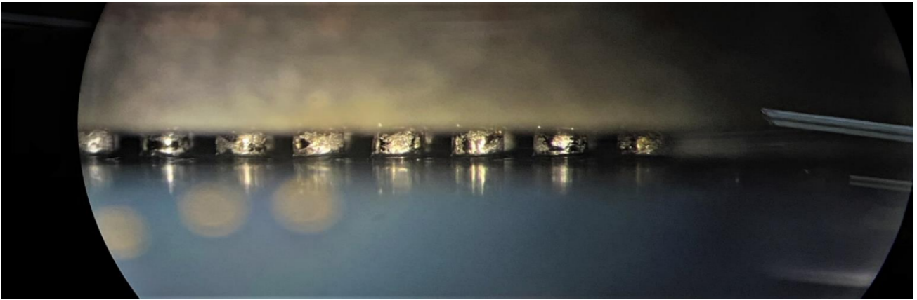
Fig. 21. Side D solder balls after rework is done by Vapor Phase Soldering.
